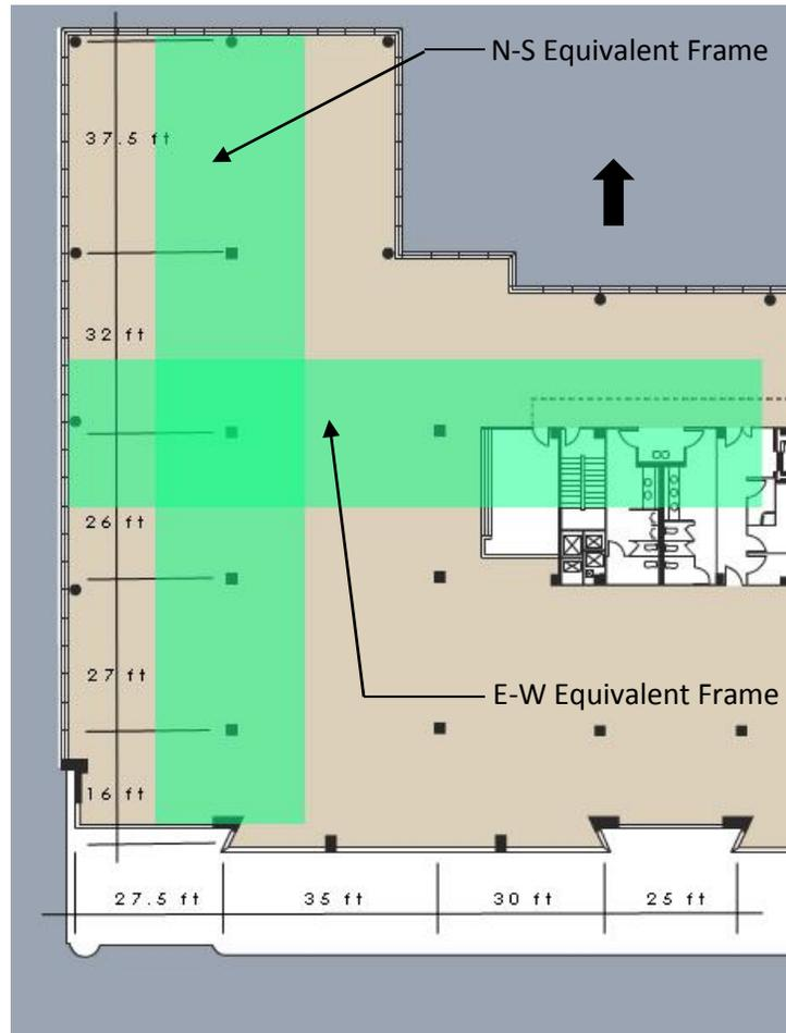
**Figure 19** Equivalent frames chosen for PT design highlighted in green
