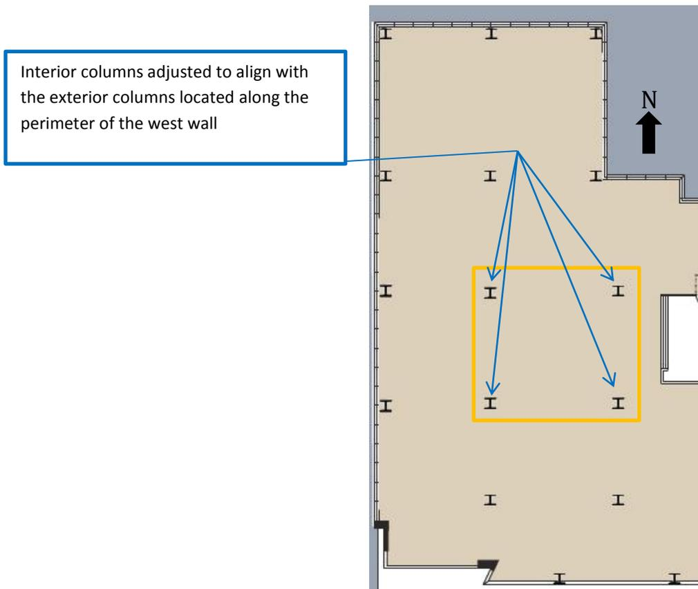
**Figure 17** Proposed steel column layout for composite steel system
