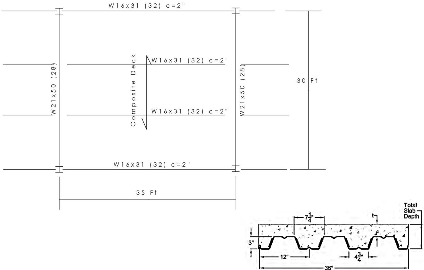
**Figure 16** Composite Steel System Layout (top left) and composite deck section taken from Vulcraft 2008 catalog (lower right)
