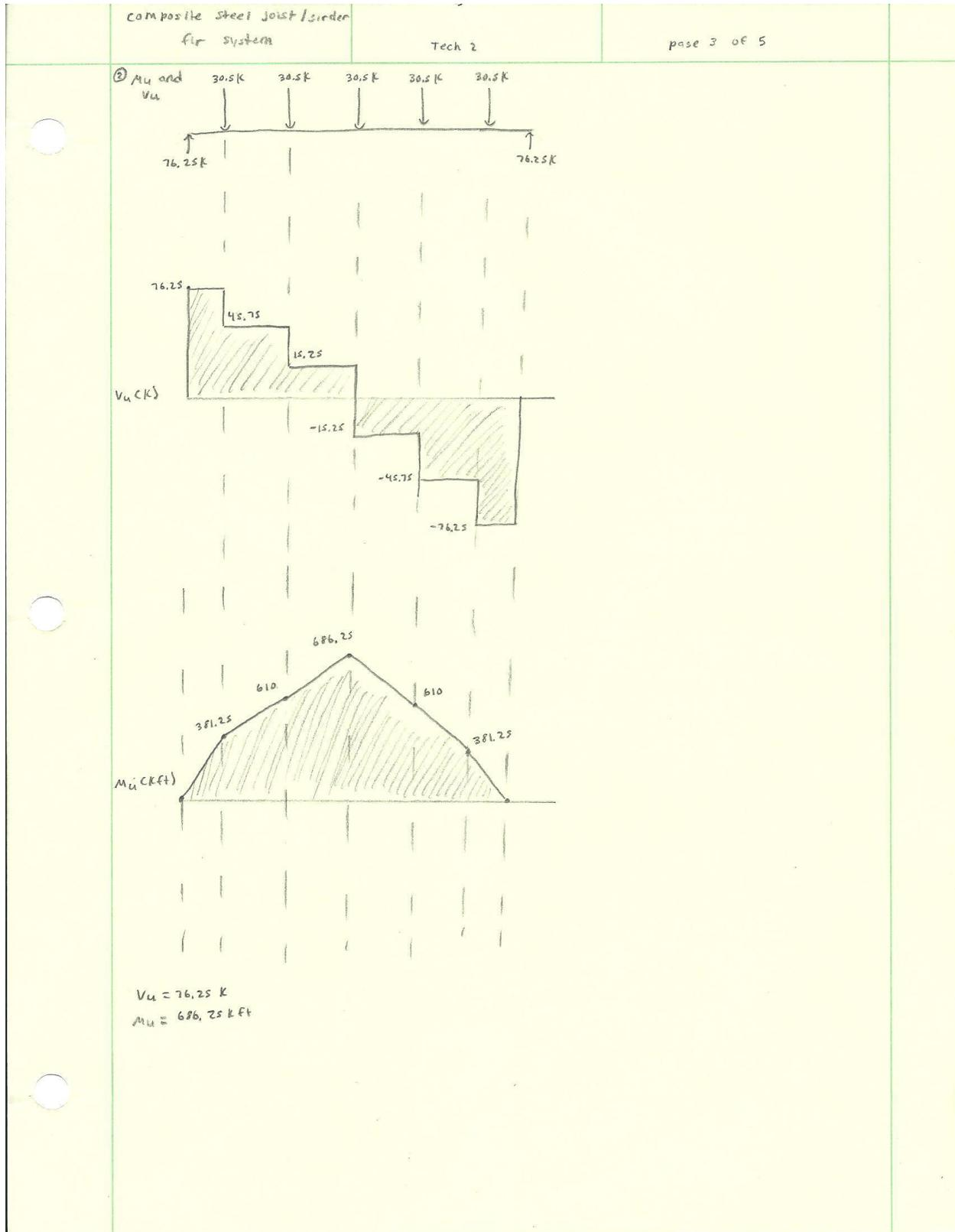
composite steel joist / girder
