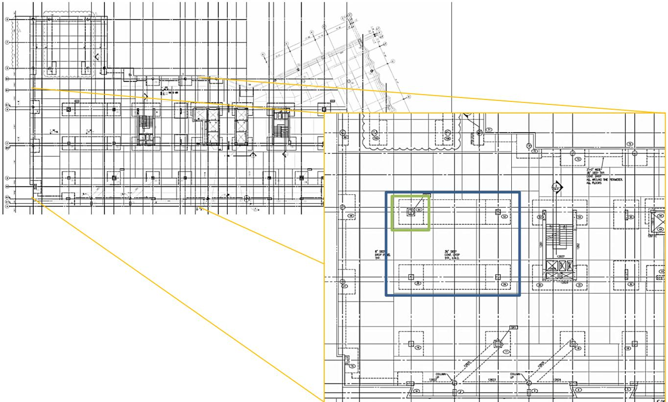
**Figure 15** Existing system typical structural layout (left) and an enlarged layout of the interior panel used for gravity spot check analyses (right)
