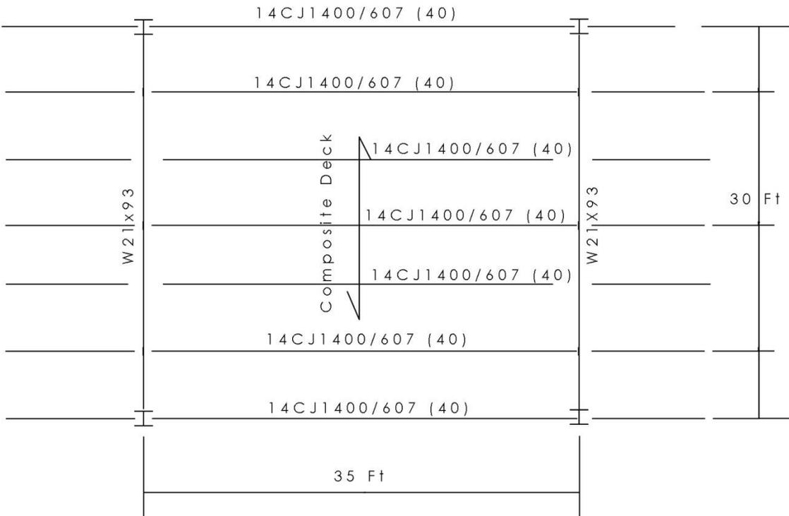
**Figure 20** composite joist/steel girder layout
