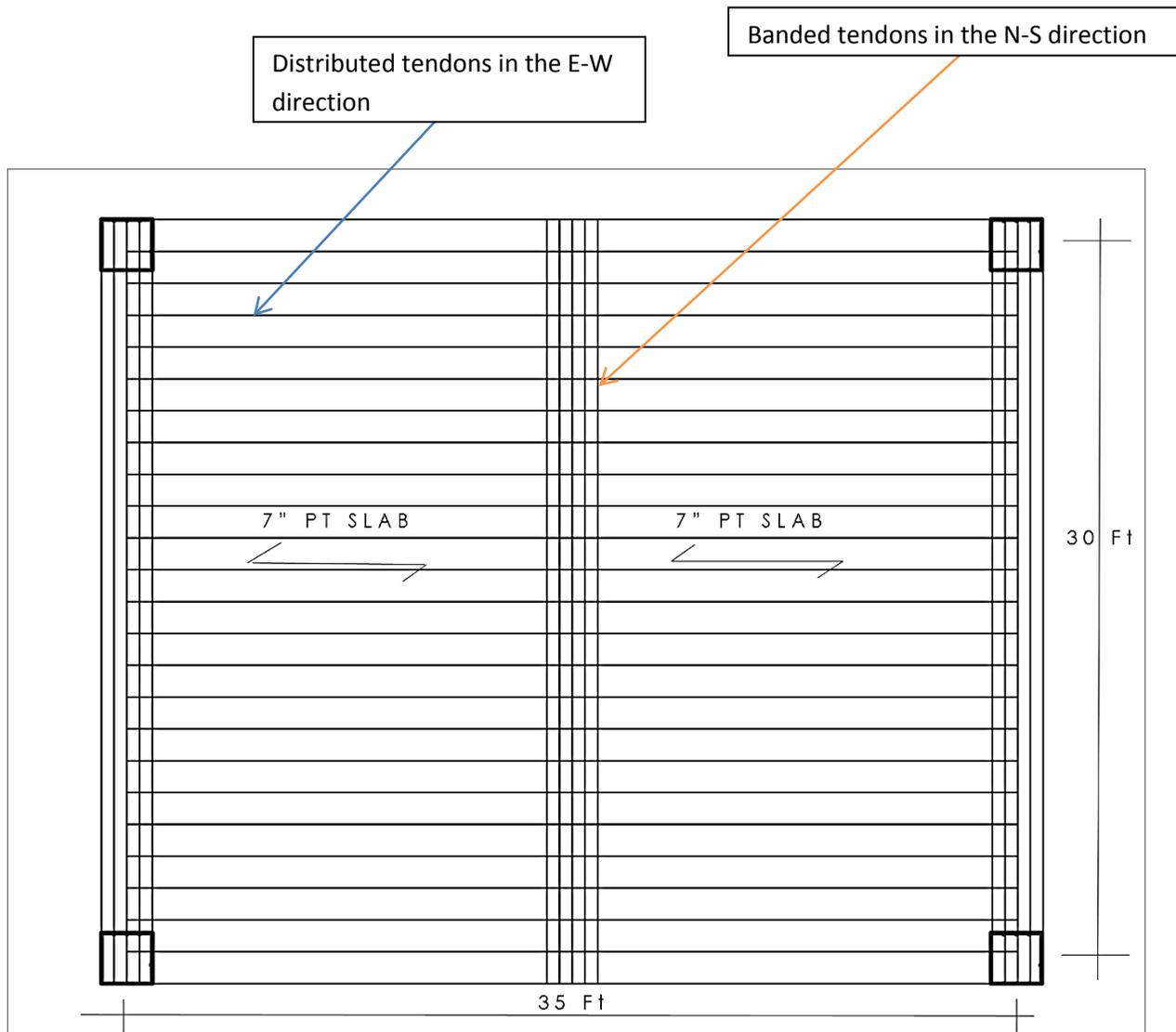
**Figure 18** post-Tension tendon layout
