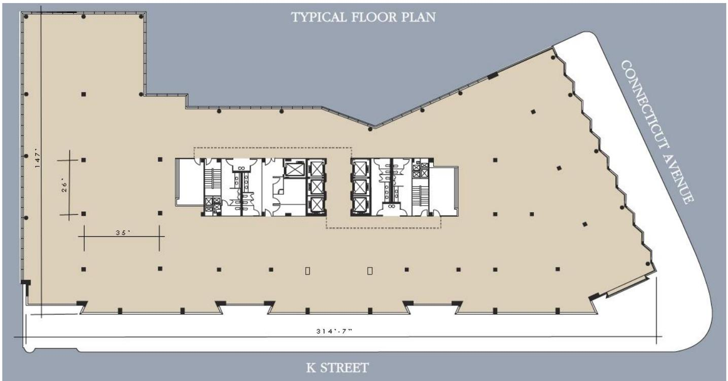
**Figure 8** Floor plan displaying column locations and bays
